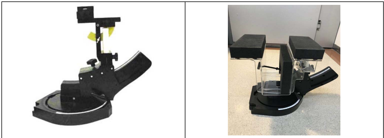
Device holder supplied by SPEAG
