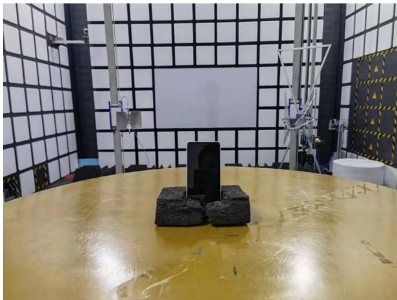
Spurious Radiated Emissions Test setup
