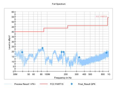
Frequency Range: 30MHz-1000 MHz Detector: QP mode
