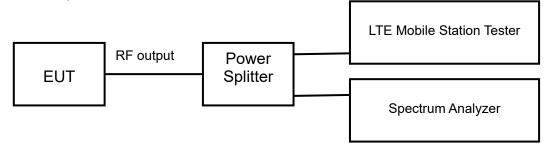
Test procedure: KDB 971168 D01 v03r01 – Section 4.2
