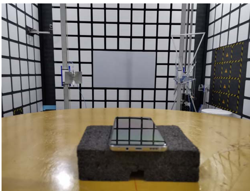
Spurious Radiated Emissions Test setup
