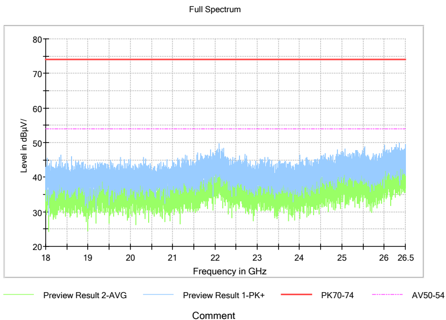
Pic14. Radiated emission (18GHz –26GHz)
