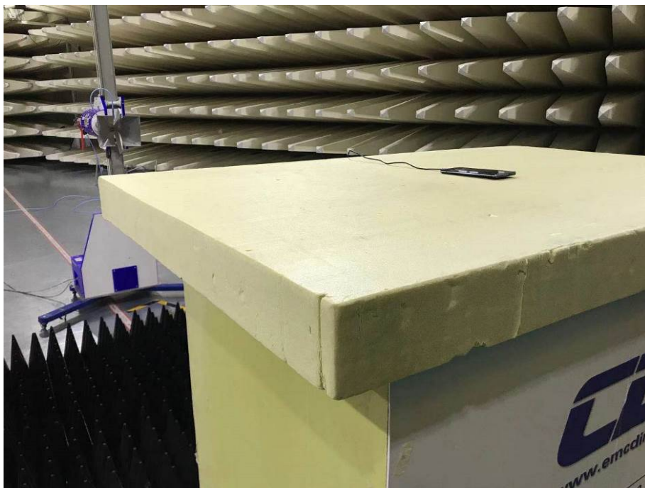
Spurious Radiated Emissions Test setup
