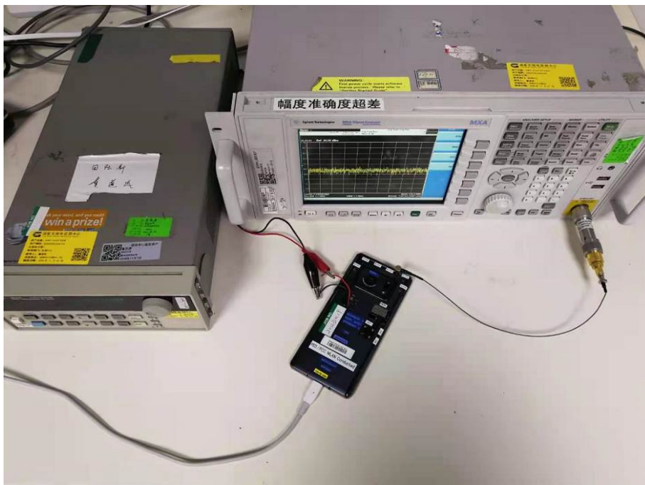
RF Conducted Test setup (BT/WIFI)
