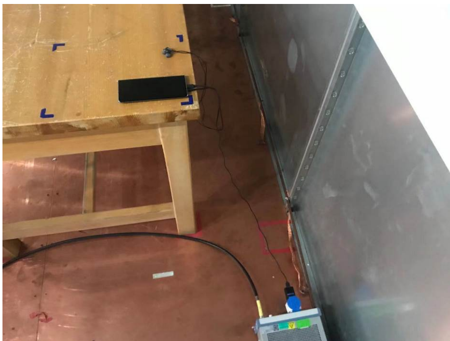
Conducted Emissions Test Setup (with charger)
