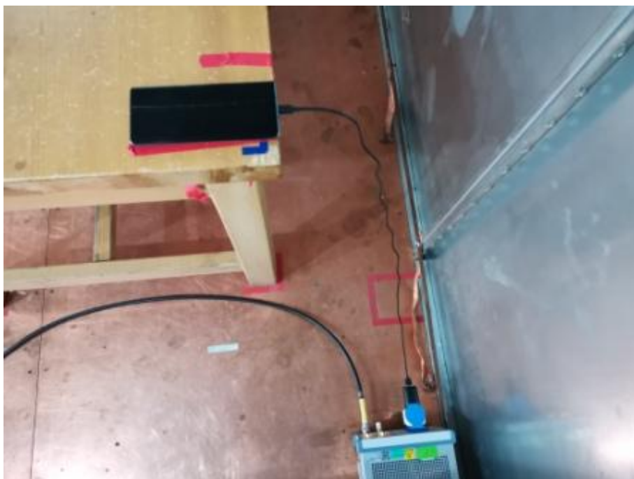
Conducted Emissions Test Setup (with charger)
