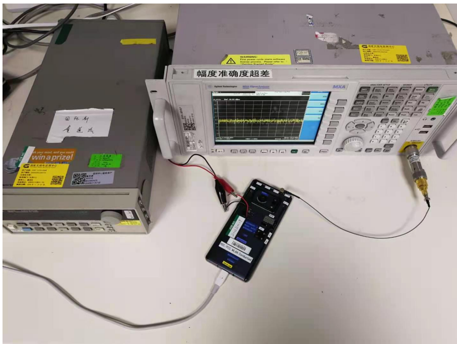
RF Conducted Test setup (BT/WIFI)
