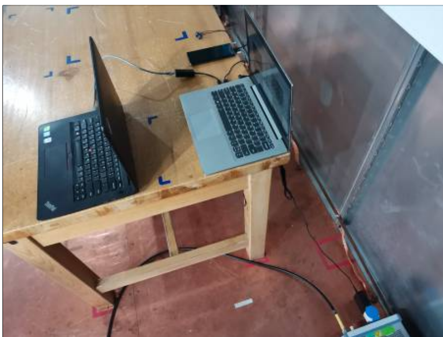
Conducted Emissions Test Setup
