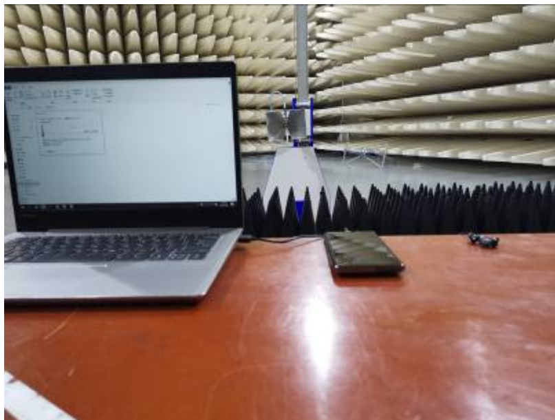
Radiated Emissions Test Setup (above 1GHz)
