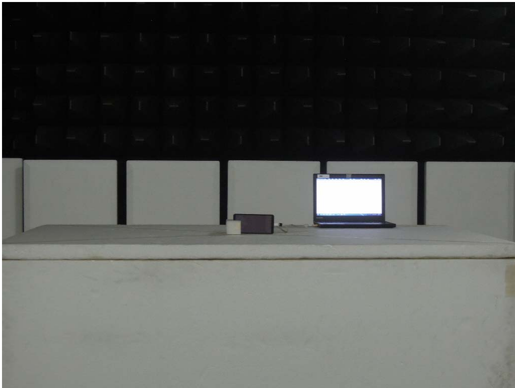
Radiated Emission Set up Photos (Front View)
