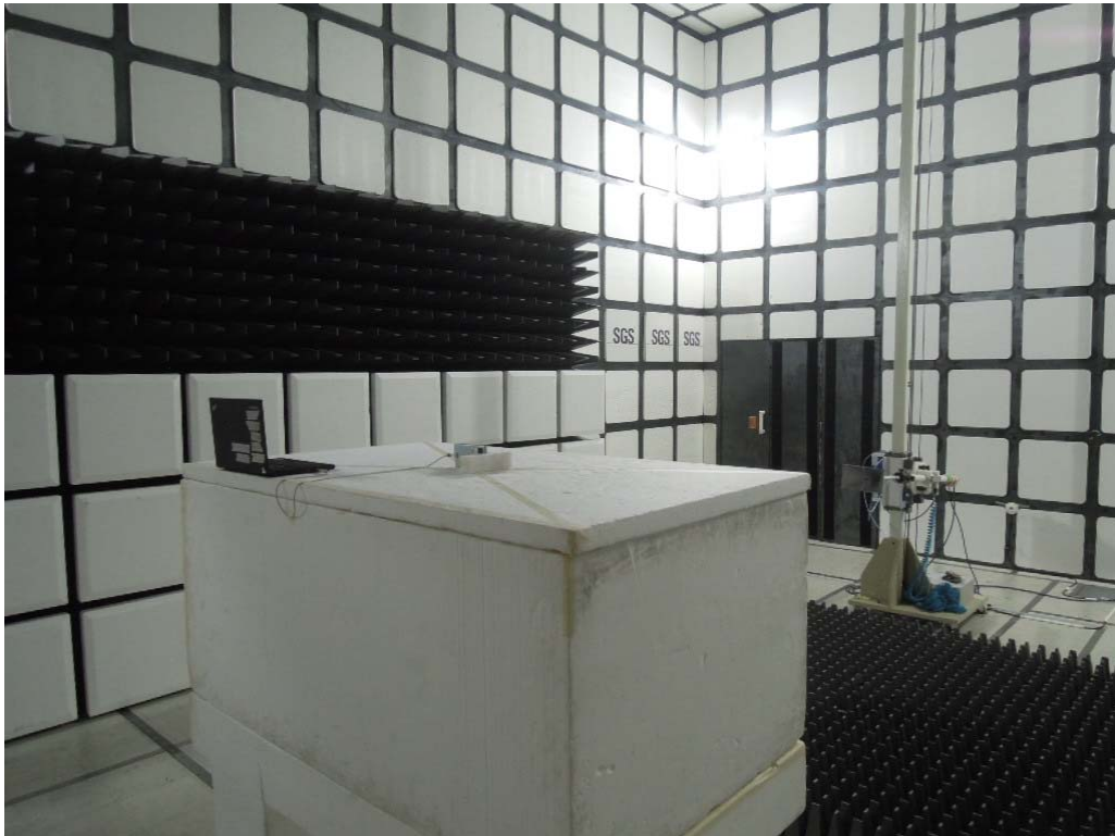
Radiated Emission Set up Photos (Front View)
