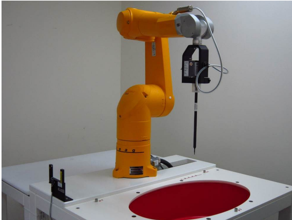
Fig.1 Photograph of the SAR measurement system
