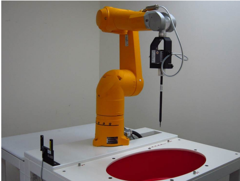
Fig.1 Photograph of the SAR measurement system
