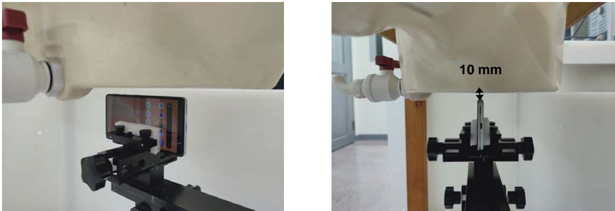
Fig.13 EUT Right side to flat phantom
