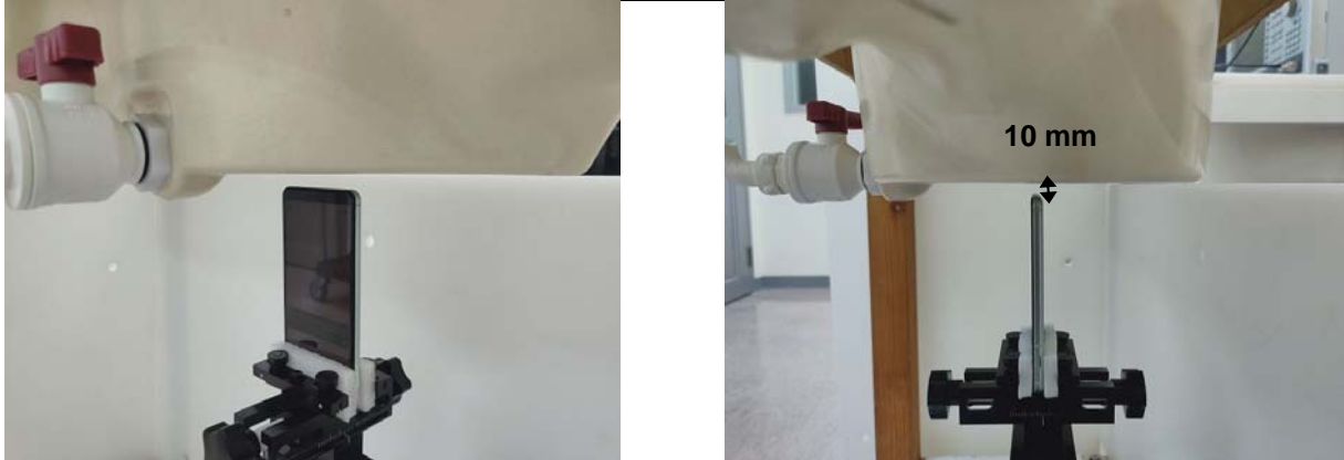
Fig.12 EUT Bottom side to flat phantom
