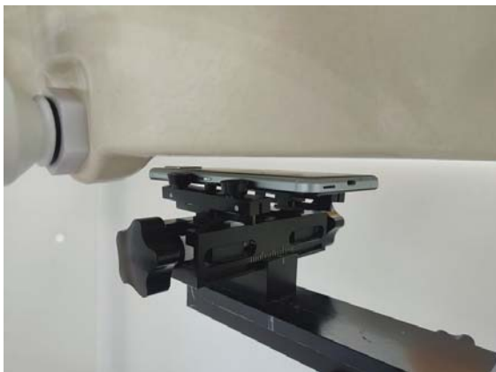
Fig.10 EUT Back side to flat phantom
