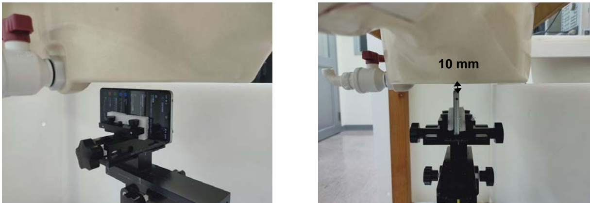
Fig.14 EUT Left side to flat phantom
