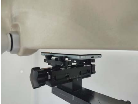
Fig.9 EUT Front side to flat phantom
