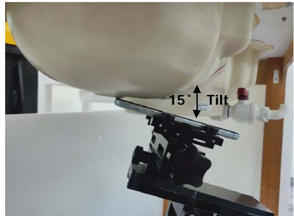
Fig.4 Right Head Section / Ear-Tilt Position(15°)
