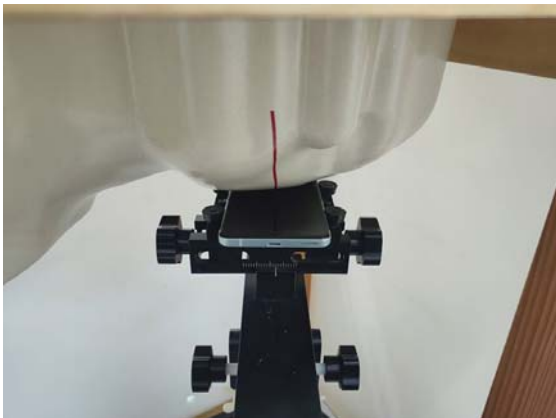
Fig.5 Left Head Section / Cheek-Touch Position
