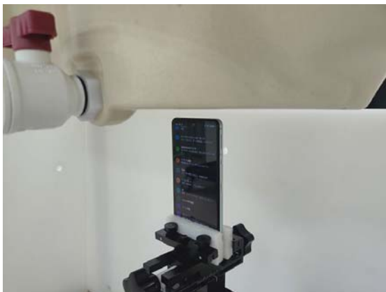
Fig.11 EUT Top side to flat phantom
