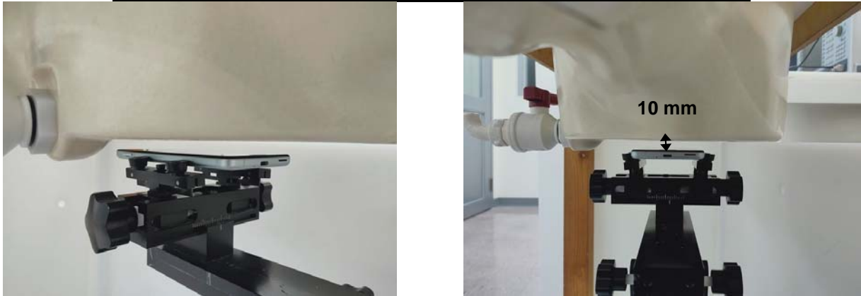
Fig.7 EUT Front side to flat phantom
