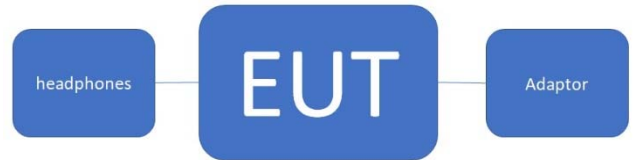
Fig. 2-3 Conducted (AC Power Line) Emission
