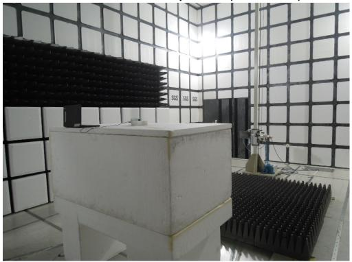
Radiated Emission Set up Photos (Front View)
