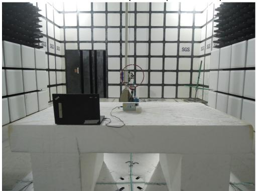
Radiated Emission Set up Photos (Below 1GHz)
