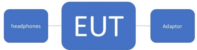
Fig 2-3 Conducted (AC Power Line) Emission
