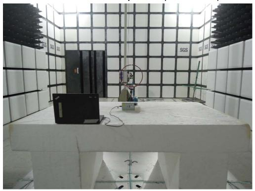
Radiated Emission Set up Photos (Below 1GHz)
