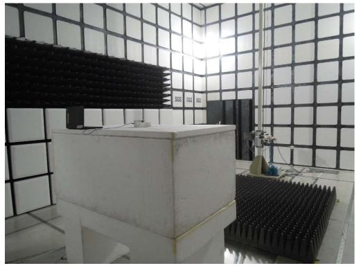
Radiated Emission Set up Photos (Front View)
