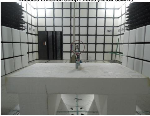
Radiated Emission Setup Photos (30MHz~1GHz)
