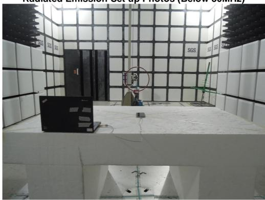
Radiated Emission Set up Photos (Below 1GHz)
