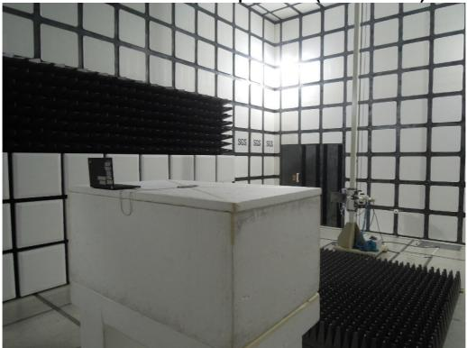
Radiated Emission Set up Photos (Front View)
