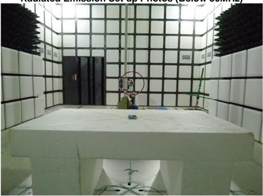
Radiated Emission Set up Photos (Below 1GHz)
