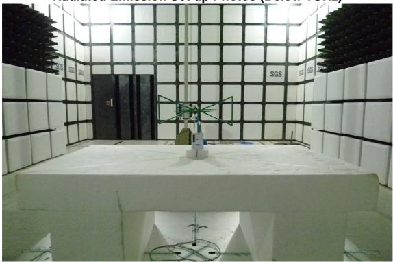
Radiated Emission Set up Photos (Above 1GHz)
