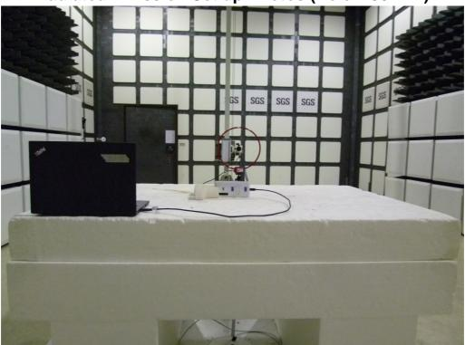
Radiated Emission Set up Photos (Below 1GHz)
