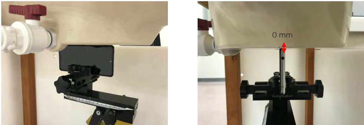
Fig.19 EUT Left side to flat phantom
