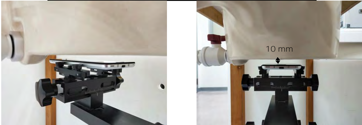
Fig.7 EUT Front side to flat phantom
