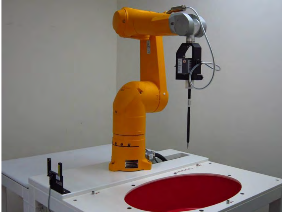
Fig.1 Photograph of the SAR measurement system
