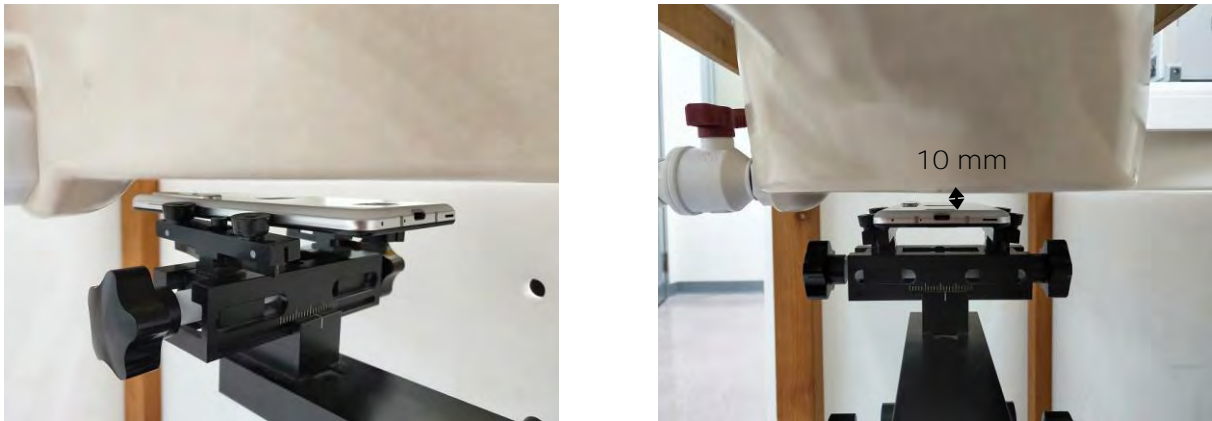
Fig.8 EUT Back side to flat phantom
