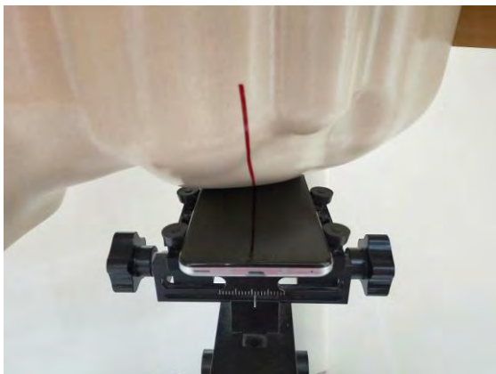
Fig.5 Left Head Section / Cheek-Touch Position
