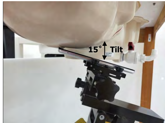
Fig.4 Right Head Section / Ear-Tilt Position(15°)
