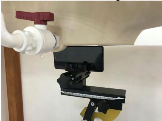
Fig.17 EUT Right side to flat phantom
