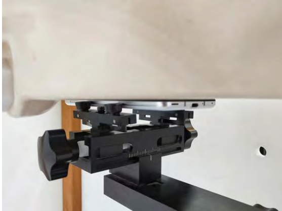
Fig.15 EUT Front side to flat phantom
