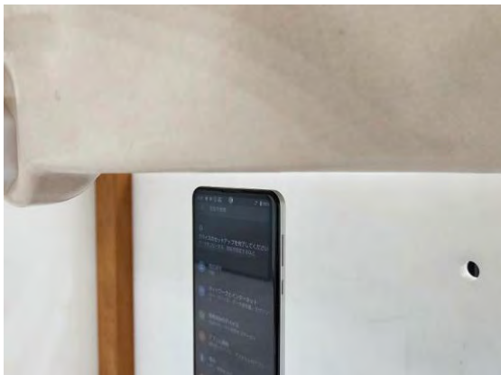
Fig.14 EUT Top side to flat phantom
