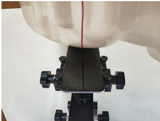
Fig.4 Right Head Section / Ear-Tilt Position(15°)
