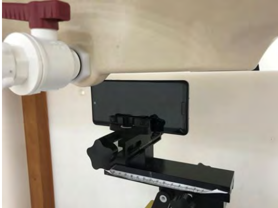
Fig.12 EUT Right side to flat phantom
