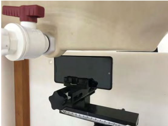
Fig.13 EUT Left side to flat phantom
