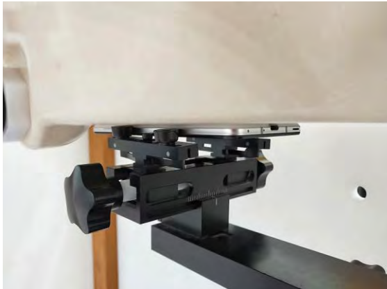
Fig.16 EUT Back side to flat phantom
