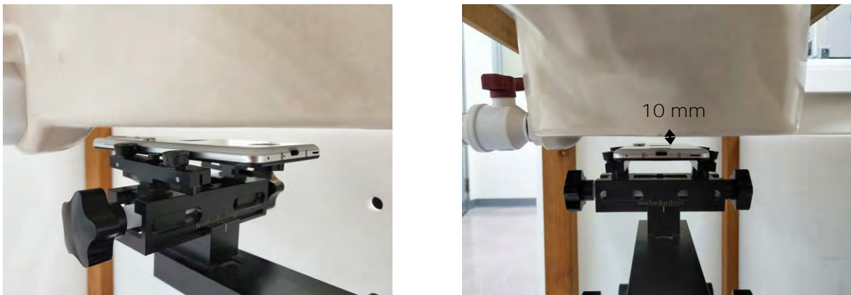
Fig.10 EUT Back side to flat phantom
