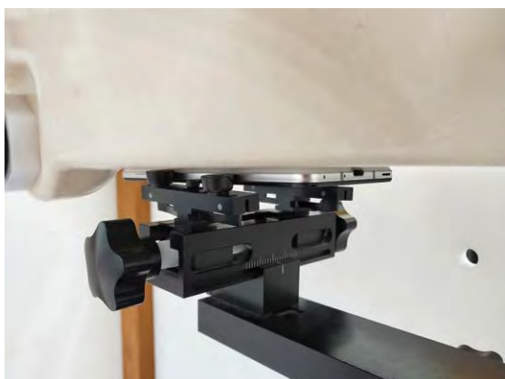
Fig.16 EUT Back side to flat phantom
