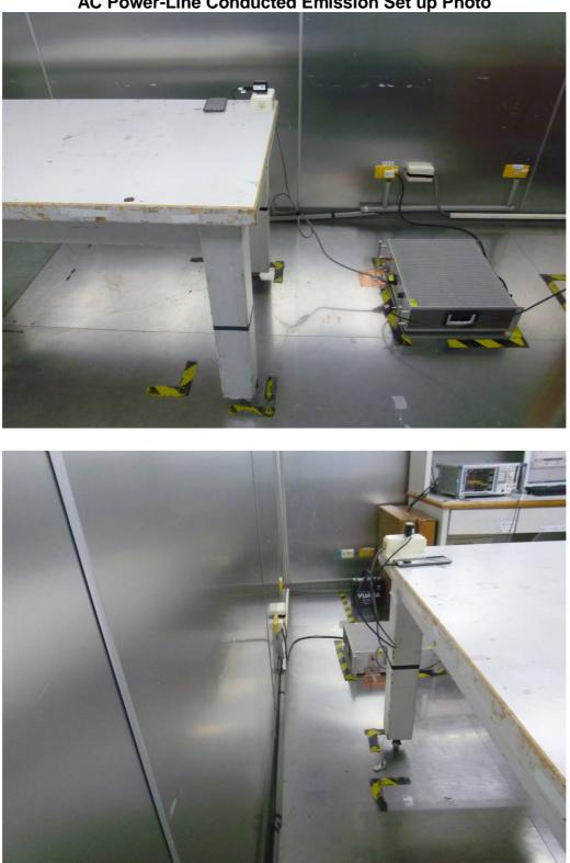
AC Power-Line Conducted Emission Set up Photo
