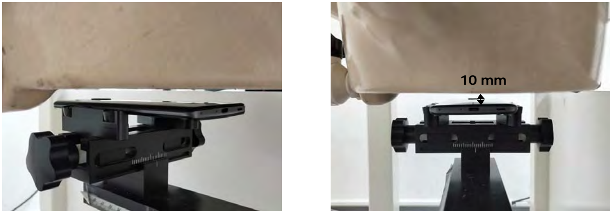
Fig.8 EUT Back side to flat phantom
