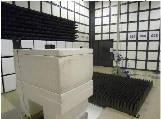
Radiated Emission Set up Photos (Front View)
