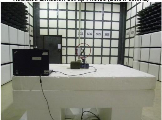
Radiated Emission Set up Photos (Below 1GHz)
