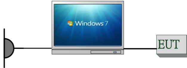
Fig. 2-1 Radiated Emission Configuration (NFC & BT & BLE & WLAN)
