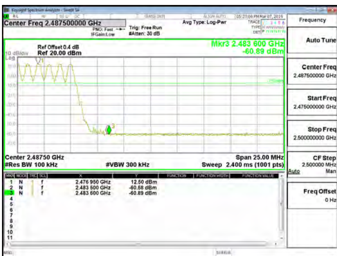
Hopping Band Edge_GFSK_1M_DH5_2480MHz
