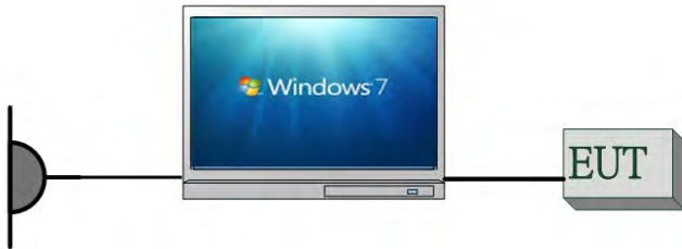
Fig. 2-2 AC Power Line Conducted Emission
