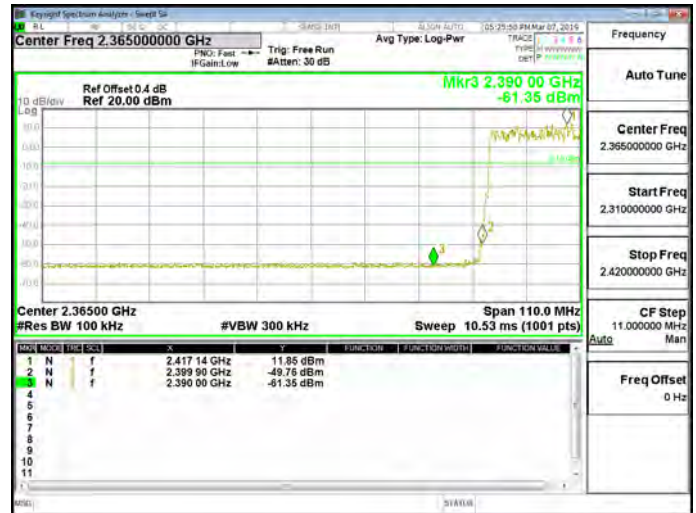
Hopping Band Edge_8DPSK_3M_DH5_2480MHz
