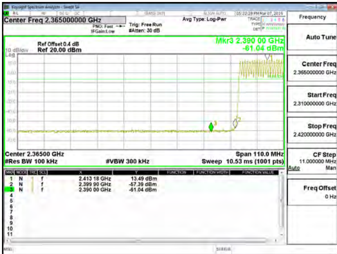
Hopping Band Edge_GFSK_1M_DH5_2480MHz
