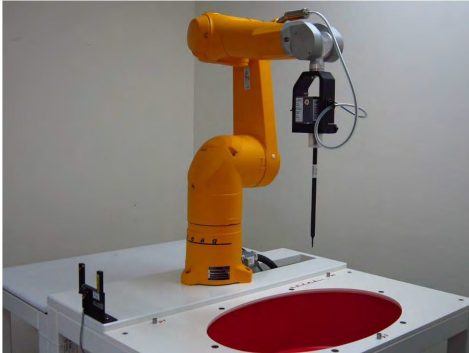
Fig.1 Photograph of the SAR measurement system
