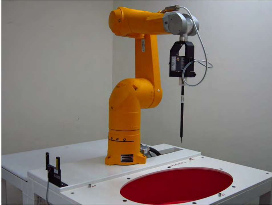
Fig.1 Photograph of the SAR measurement system
