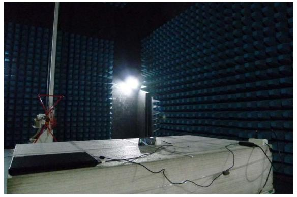
Radiated Emission Set up Photos (Above 1GHz)
