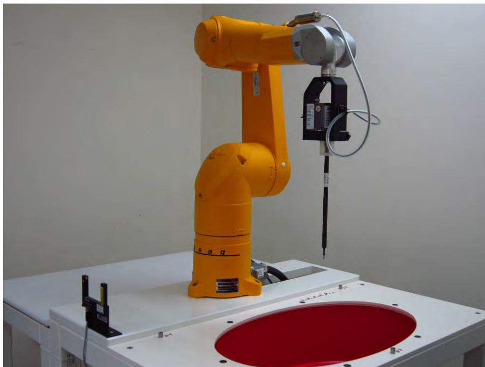
Fig.1 Photograph of the SAR measurement system
