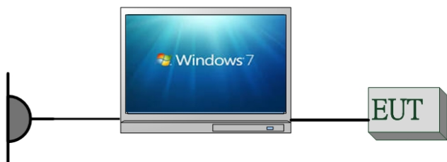
Fig. 2-2 AC Power Line Conducted Emission
