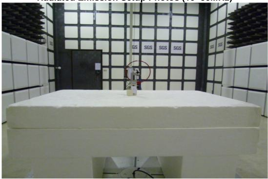
Radiated Emission Setup Photos (30MHz~1GHz)
