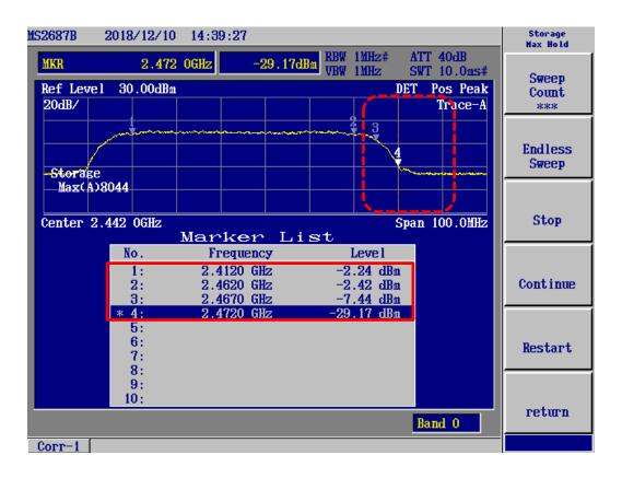
1-11ch = Enabled 12-13ch = Disabled ⇒ Operation Check Result = OK
