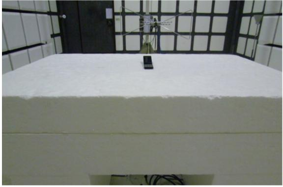
Radiated Emission Set up Photos (Above 1GHz)
