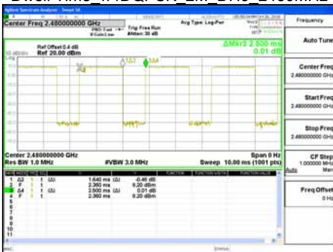
Dwell Time \pi 4DQPSK 2M DH3 2480MHz
