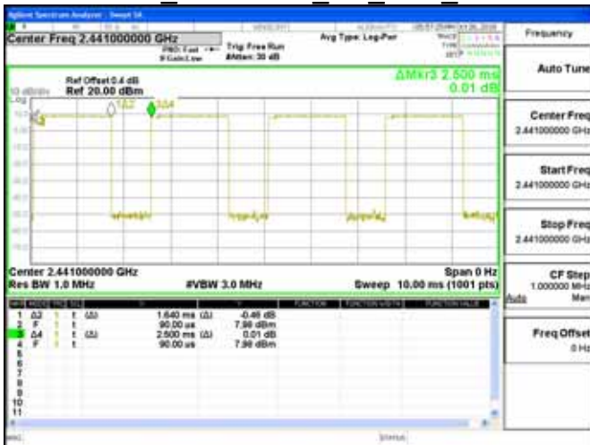
Dwell Time \pi 4DQPSK 2M DH3 2480MHz
