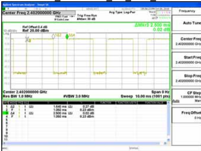
Dwell Time \pi 4DQPSK 2M DH3 2441MHz
