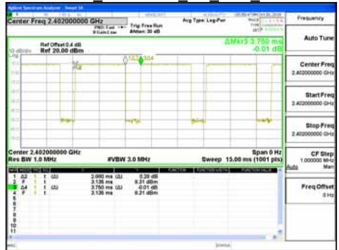
Dwell Time \pi 4DQPSK 2M DH5 2441MHz
