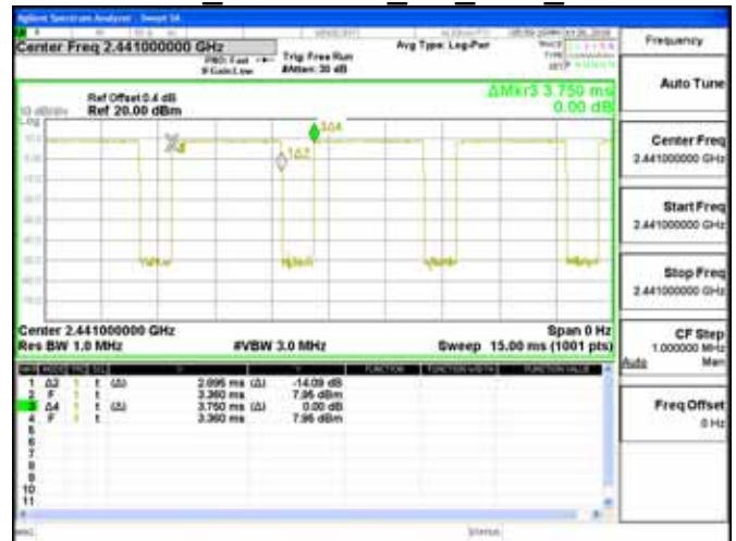
Dwell Time \pi 4DQPSK 2M DH5 2480MHz
