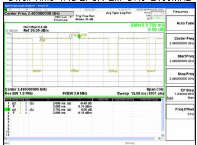
Dwell Time \pi 4DQPSK 2M DH5 2480MHz
