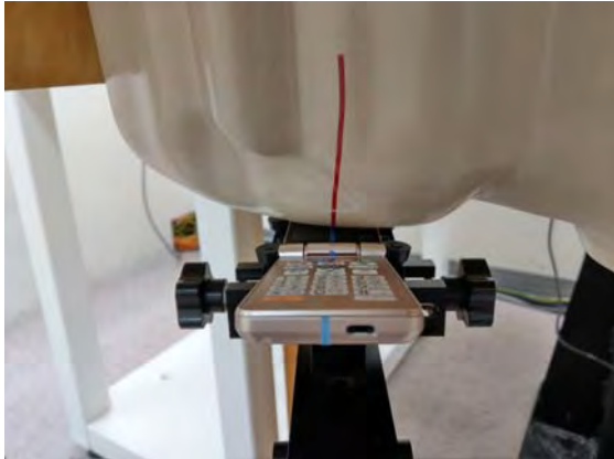
Fig.3 Right Head Section / Cheek-Touch Position
