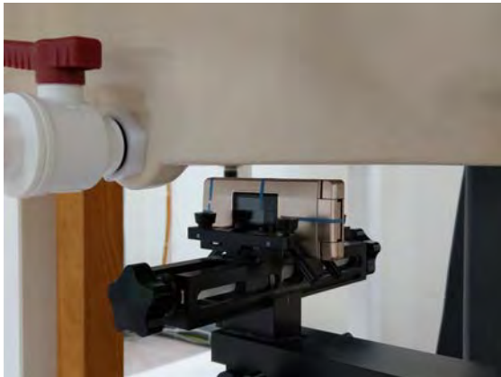
Fig.13 EUT Left side to flat phantom
