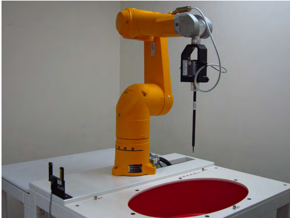
Fig.1 Photograph of the SAR measurement system
