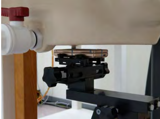
Fig.7 EUT Front side to flat phantom
