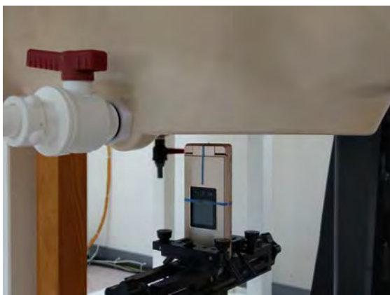
Fig.11 EUT Top side to flat phantom
