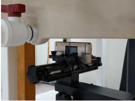
Fig.12 EUT Right side to flat phantom
