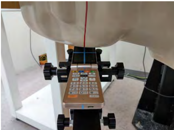
Fig.4 Right Head Section / Ear-Tilt Position(15°)
