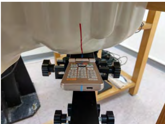
Fig.5 Left Head Section / Cheek-Touch Position
