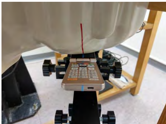
Fig.5 Left Head Section / Cheek-Touch Position
