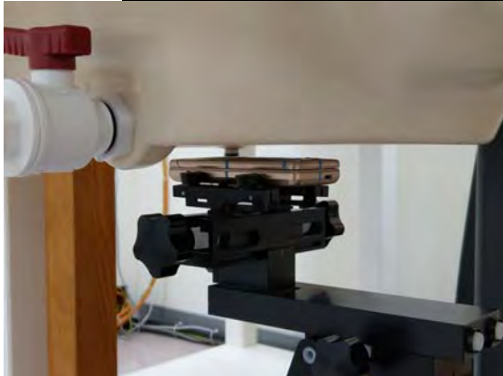
Fig.9 EUT Front side to flat phantom
