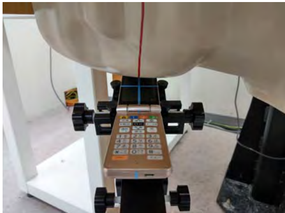
Fig.4 Right Head Section / Ear-Tilt Position(15°)
