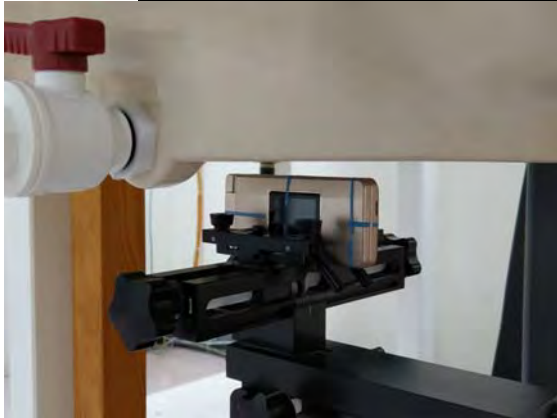
Fig.12 EUT Right side to flat phantom
