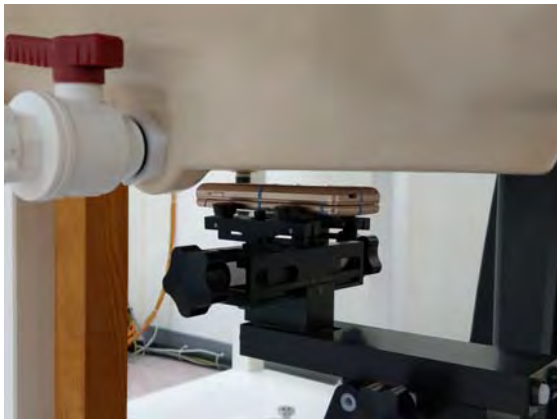
Fig.10 EUT Back side to flat phantom
