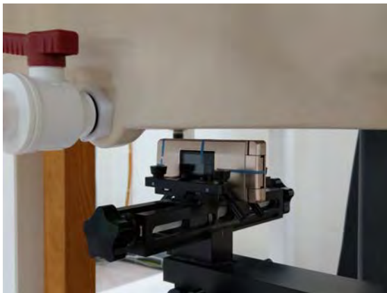
Fig.13 EUT Left side to flat phantom
