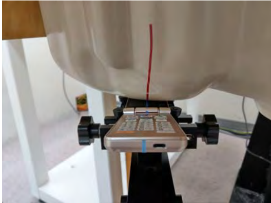
Fig.3 Right Head Section / Cheek-Touch Position
