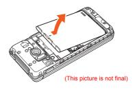
Using unnecessary force when attaching or removing the battery pack may damage the connector terminal on the handset.
