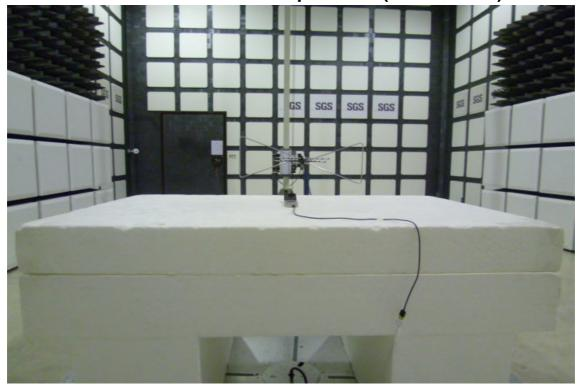
Radiated Emission Set up Photos (Above 1GHz)
