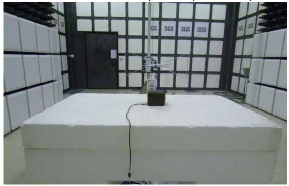
Radiated Emission Set up Photos (Above 1GHz)
