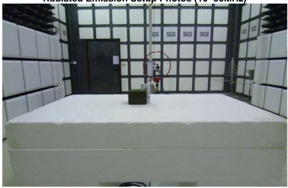
Radiated Emission Setup Photos (30MHz~1GHz)
