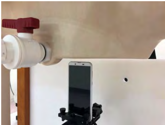
Fig.11 EUT Top side to flat phantom
