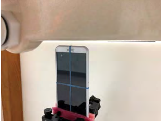
Fig.12 EUT Bottom side to flat phantom
