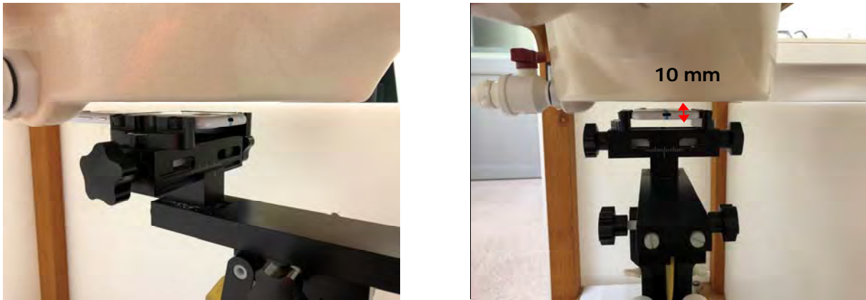
Fig.8 EUT Back side to flat phantom
