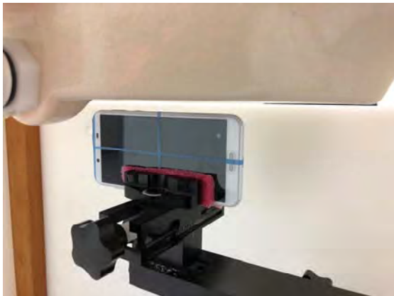
Fig.13 EUT Right side to flat phantom
