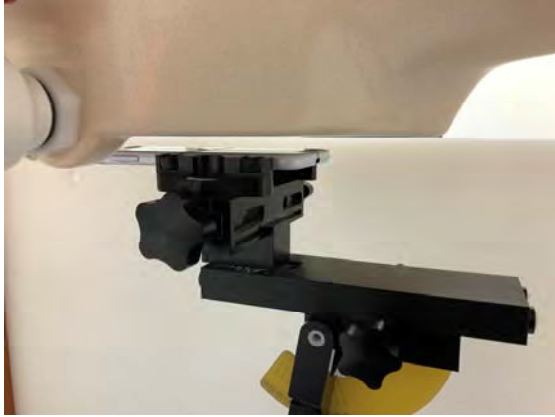
Fig.9 EUT Front side to flat phantom
