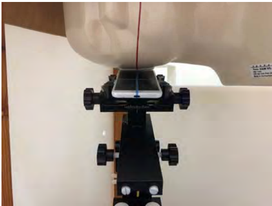
Fig.4 Right Head Section / Ear-Tilt Position(15°)
