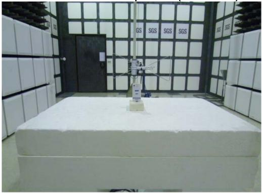
Radiated Emission Set up Photos (Above 1GHz)
