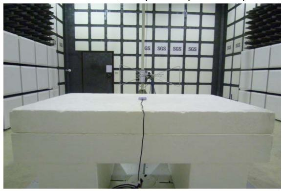
Radiated Emission Set up Photos (Above 1GHz)
