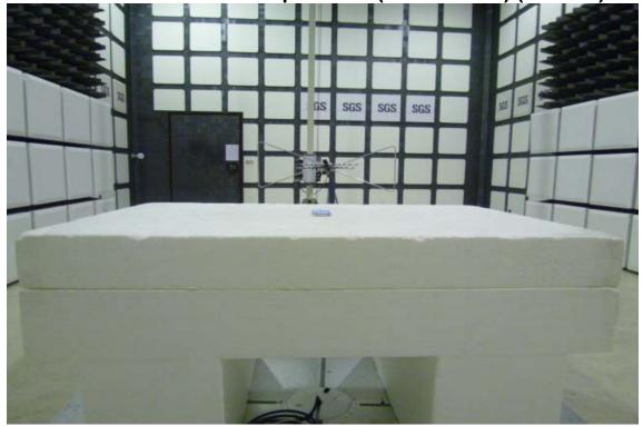
Radiated Emission Set up Photos (Above 1GHz)
