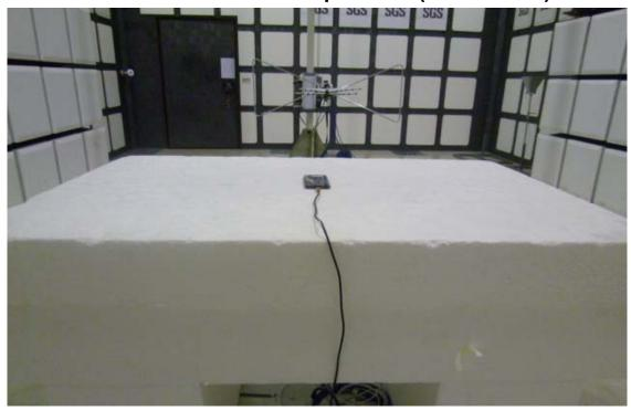
Radiated Emission Set up Photos (Above 1GHz)
