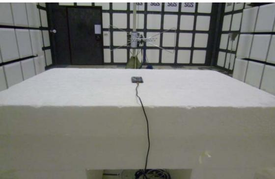
Radiated Emission Set up Photos (Above 1GHz)
